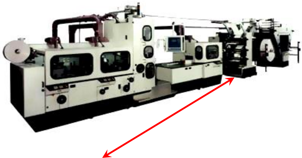
WD 627 - CI - (CENTRAL IMPRESSION UNIT) FOLDING MACHINE
