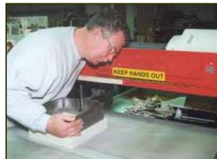
Die cutting out the blanks
