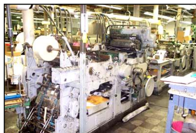
Die cutting out the blanks
